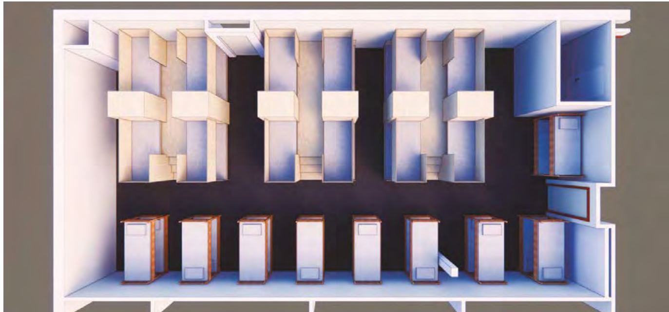
The Step-Up bedding system allows for double-height occupancy with storage and privacy. Images show standing view (top) and bird's eye (bottom) view of the Step-Up system compared to traditional bunks.
